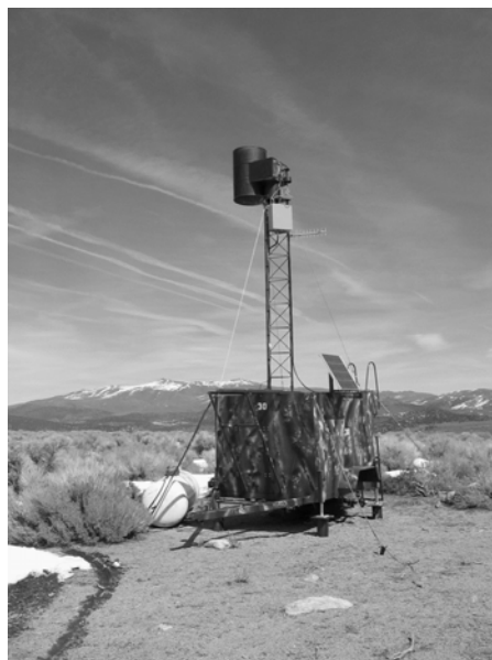
Figure 2 - Dynamo Site – ground based cloud seeding site.
